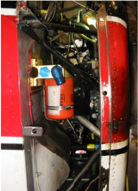
ALTERNATE ACCEPTABLE MOUNTING LOCATION FOR AIRCRAFT WITH MILITARY STYLE EXHAUST SYSTEMS.
