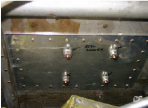
ADDITIONAL DOUBLER FIELD MADE FROM .090 6061-T6 VIEWED FROM BACKSIDE OF FIREWALL
