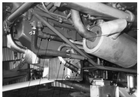
SECURE OIL LINES TO VERTICAL MOUNT WITH ADEL CLAMPS (9) & (10)
