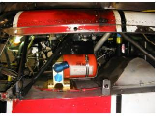
ALTERNATE ACCEPTABLE MOUNTING LOCATION FOR AIRCRAFT WITH MILITARY STYLE EXHAUST SYSTEMS.
