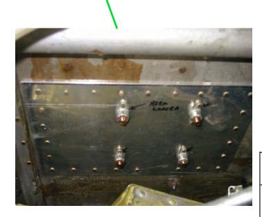
Additional doubler field made from .090 6061-T6 Viewed from backside of firewall
