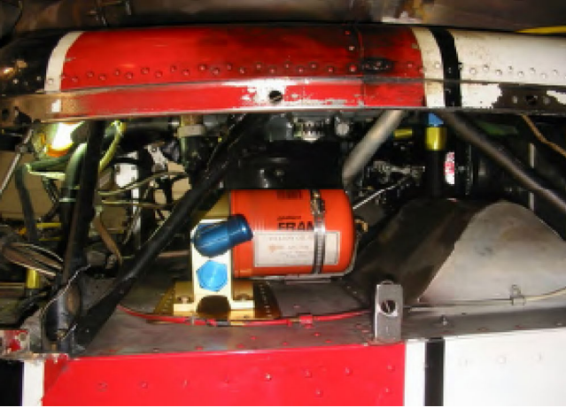
ALTERNATE ACCEPTABLE MOUNTING LOCATION FOR AIRCRAFT WITH MILITARY STYLE EXHAUST SYSTEMS.
