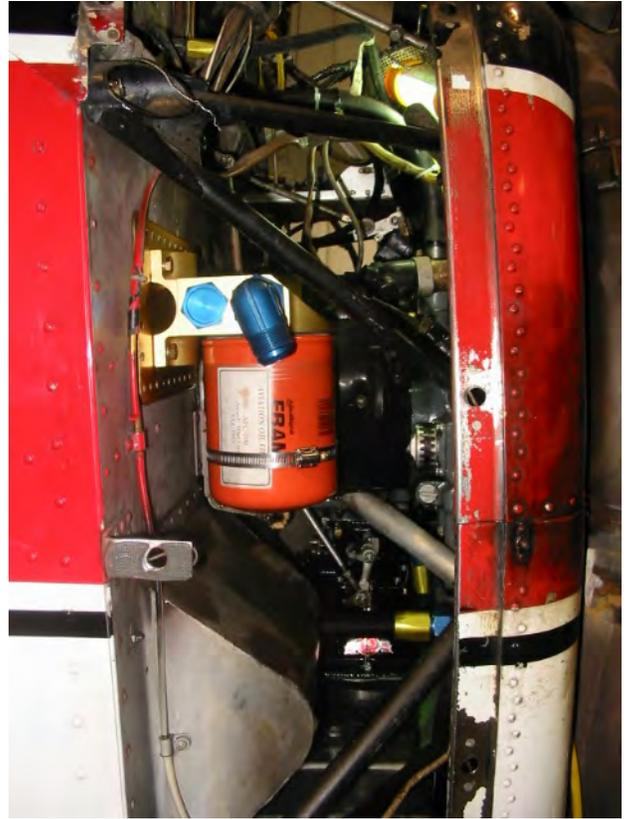
Alternate acceptable mounting location for aircraft with military style exhaust systems.
